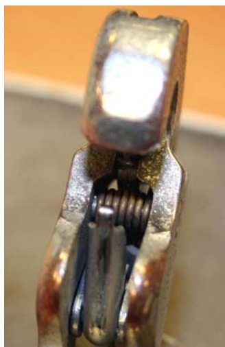
Fig 2 Identification of black double tang torsion spring (not subject to this Service Bulletin)
