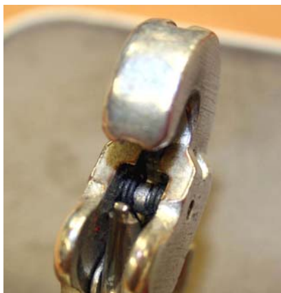
Fig 2 Identification of black double tang torsion spring (not subject to this Service Bulletin)
